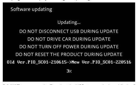
**DO NOT** turn your unit off or eject the USB storage device while the firmware is being updated.
