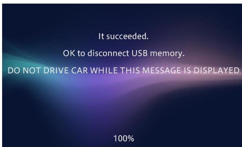
A pop sound will occur when connecting to an external amplifier after the "Update succeeded" screen is displayed; this is not a malfunction.
